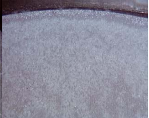
723952A disk at 50x (no mark in paint coating)
